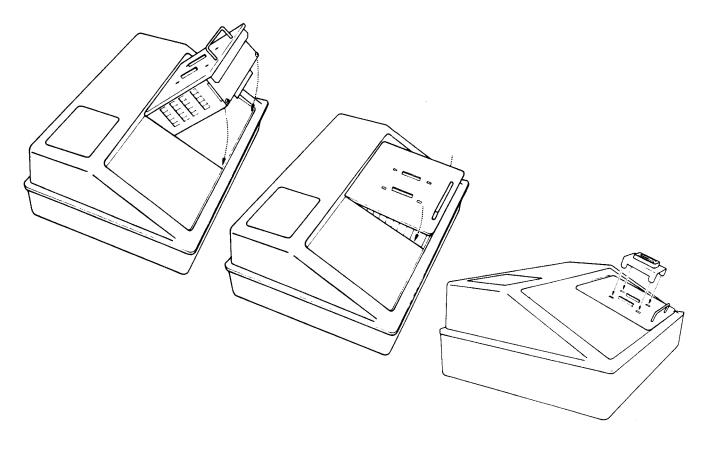
Figure 2-1. Programming Module and Socket Adapter Installation
